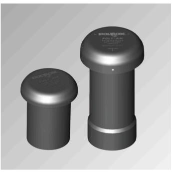
Finished landscaping should be maintained six inches below the top of the vented access cover and graded to drain runoff away from the cover. Do not obstruct the vent or allow plants, shrubbery, mulch or landscaping of any type to restrict the flow of air to the perimeter vent.
