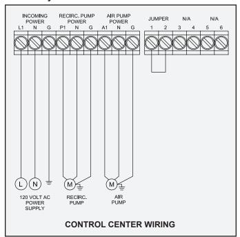
Wire from a dedicated breaker in the main service panel to the "INCOMING POWER" terminal marked "L1" in the control center using the black wire. Wire from the neutral in the main service panel to the "N" terminal using the white wire. Wire from the ground lug in the main service panel to the "G" terminal using the bare copper wire. IMPORTANT: Never allow the neutral and ground leads to be spliced/connected to common terminals.
